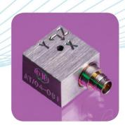
lightweight tri-axial vibration Α transducer comprising of three charge output Konic shear piezoelectric sensing elements mounted orthogonally within a block with fully titanium construction. The AT/04 is based upon the A/24 single axis sensing element and maybe considered as an alternative to the A/31 or A/34. However, the latter by virtue of being a grouping of single axis devices, are repairable and in addition the physical separation of the cable leads to visible signal axis traceability.
