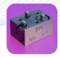
Triaxial vibration transducer comprising of three independent charge output piezo-electric accelerometers mounted orthogonally within a titanium block and welded construction with each axis is calibrated individually. It makes use of the Konic shear sensing elements to ensure a and repeatable rugged triaxial measurement under the most extreme conditions.
