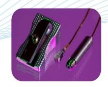
Ultra-miniature, in-line voltage output, all welded, piezo-ceramic shear plate sensing element. The low mass of the A/128/V renders it transparent in the vast majority of light weight structure vibration measurement applications.
