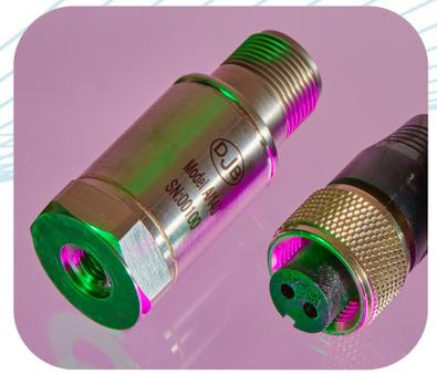
Low cost general purpose top-entry IEPE industrial accelerometer with isolated AC output and internal shielding. Manufactured in stainless steel throughout for long term vibration analysis in harsh environments. Sealed to IP67 and includes 2-pin MIL-C-5015 military style connector.
