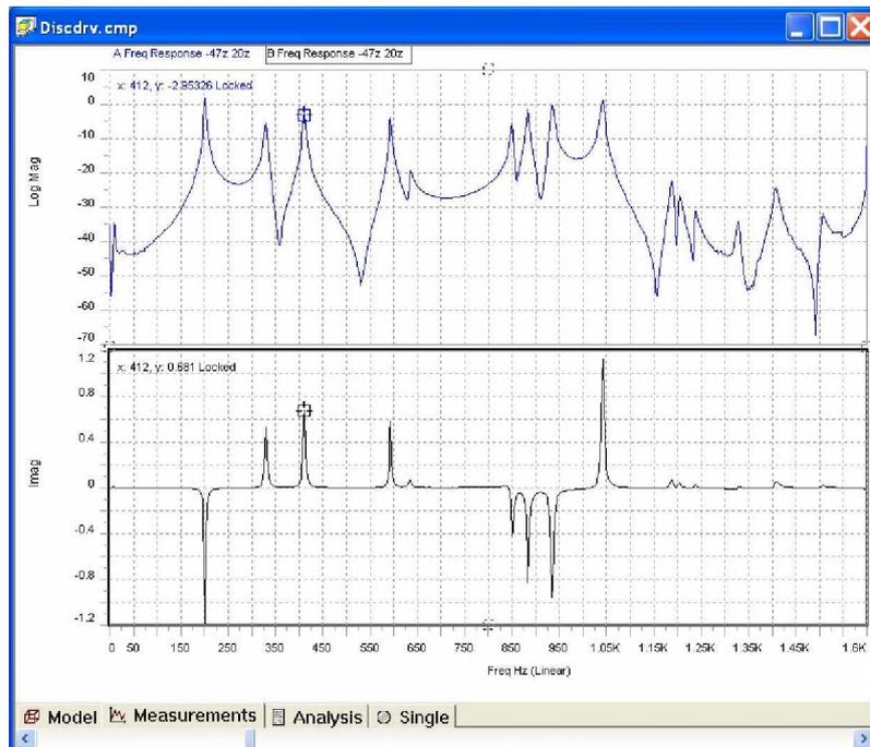
**Fig. 34 Measured Cross FRF shown as Log Magnitude & Imaginary Part**
