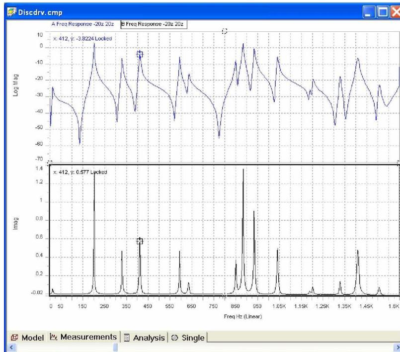
**Fig. 33 Measured Driving Point FRF shown as Log Magnitude & Imaginary Part**
