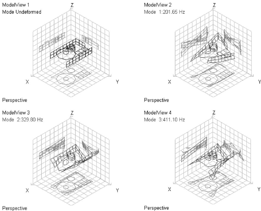
**Fig. 22 Simultaneous projection and animation of undeformed test structure and first 3 modes onto coordinate axes.**
