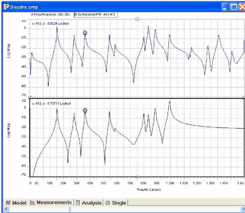
**Fig. 35 Log Magnitude FRF for Measured (20) and Synthesized (47) Driving Points**
