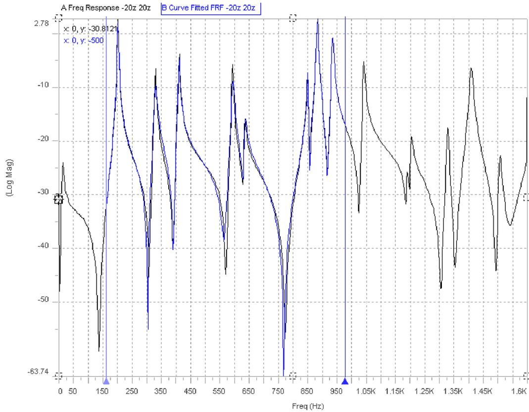
**Fig. 12; Overlay of curve-fit of 8 resonances with test data**
