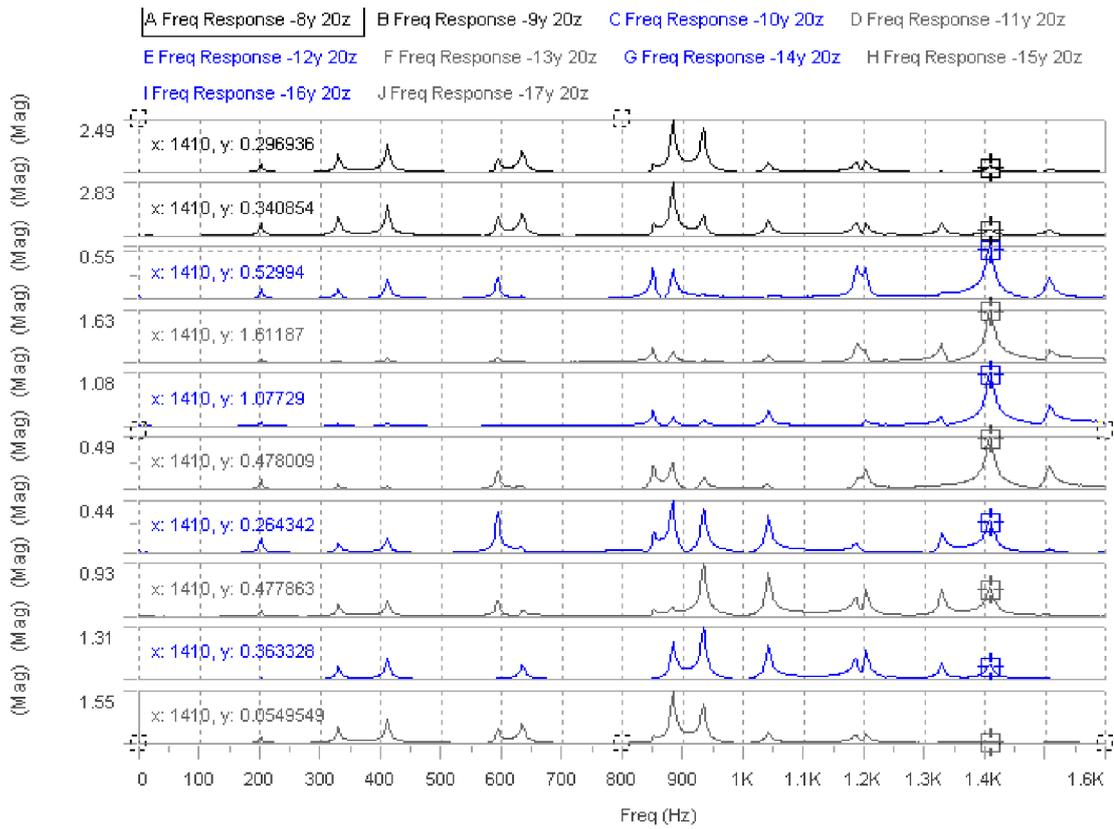
**Fig. 8; Cascade of 10 FRF's shown in Linear Magnitude format**
