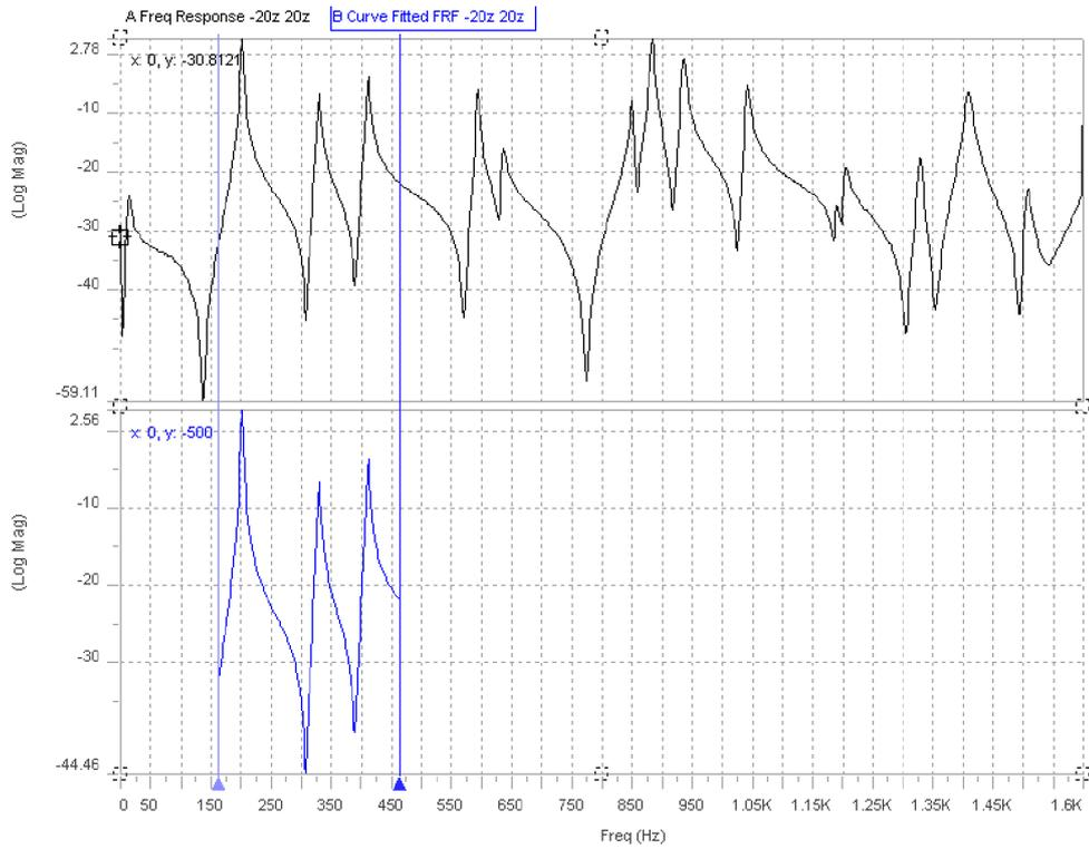
**Fig. 10; Curve-fit of first 3 resonances shown tiled with full Driving Point FRF**
