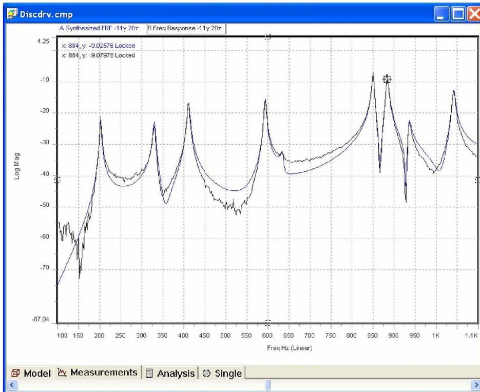
**Fig. 31 Overlay of Measured and Synthesized FRF for -11Y, 20Z**
