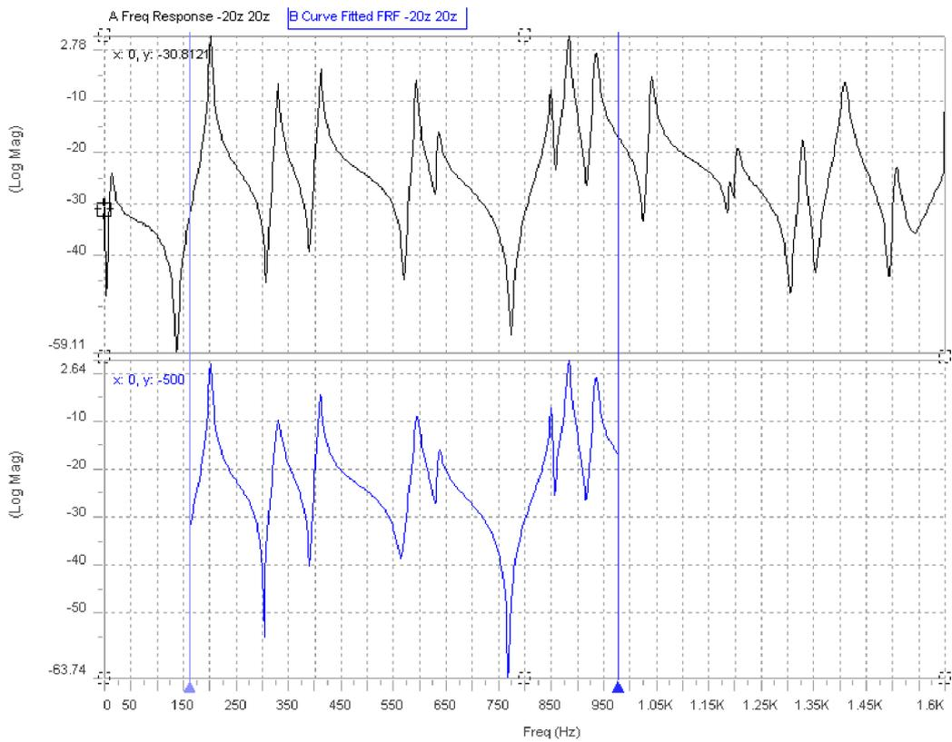
**Fig. 11; Curve-fit of first 8 resonances shown tiled with full Driving Point FRF**
