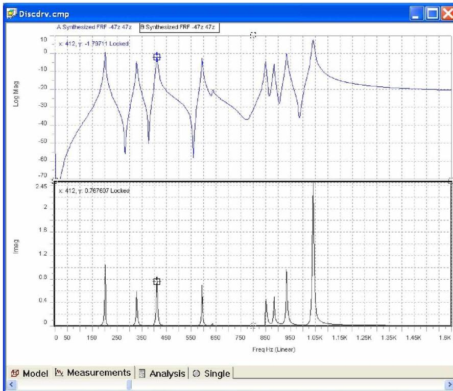
**Fig. 35 Synthesized Driving Point FRF for location 47Z**
