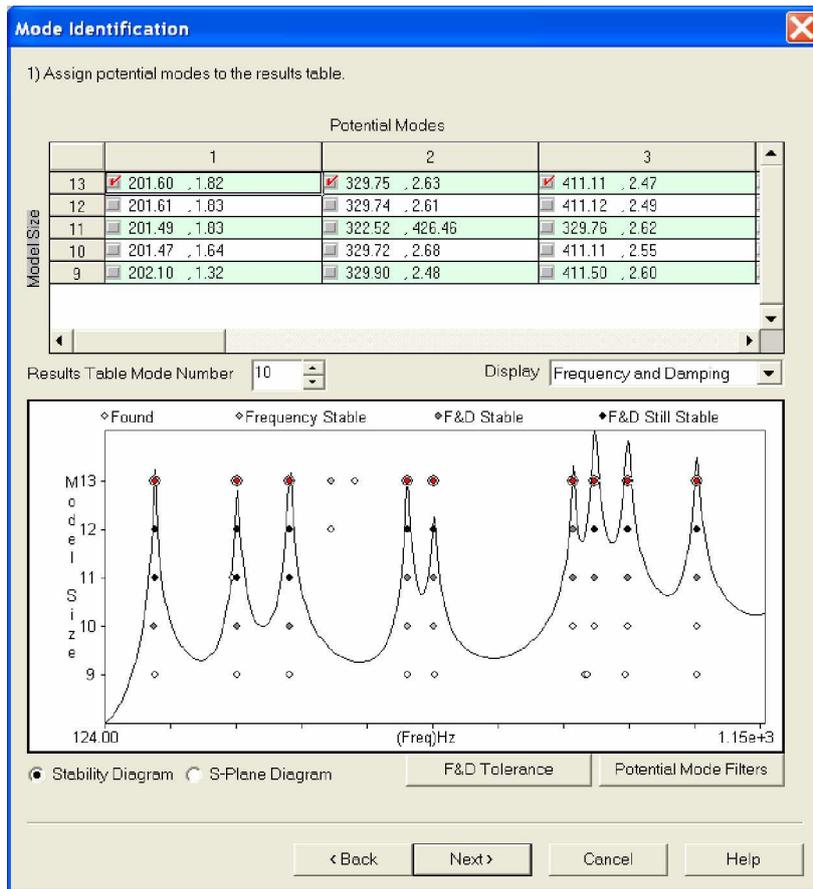
Fig. 14; Setting up Stability Diagram as part of Modal Identification Function
