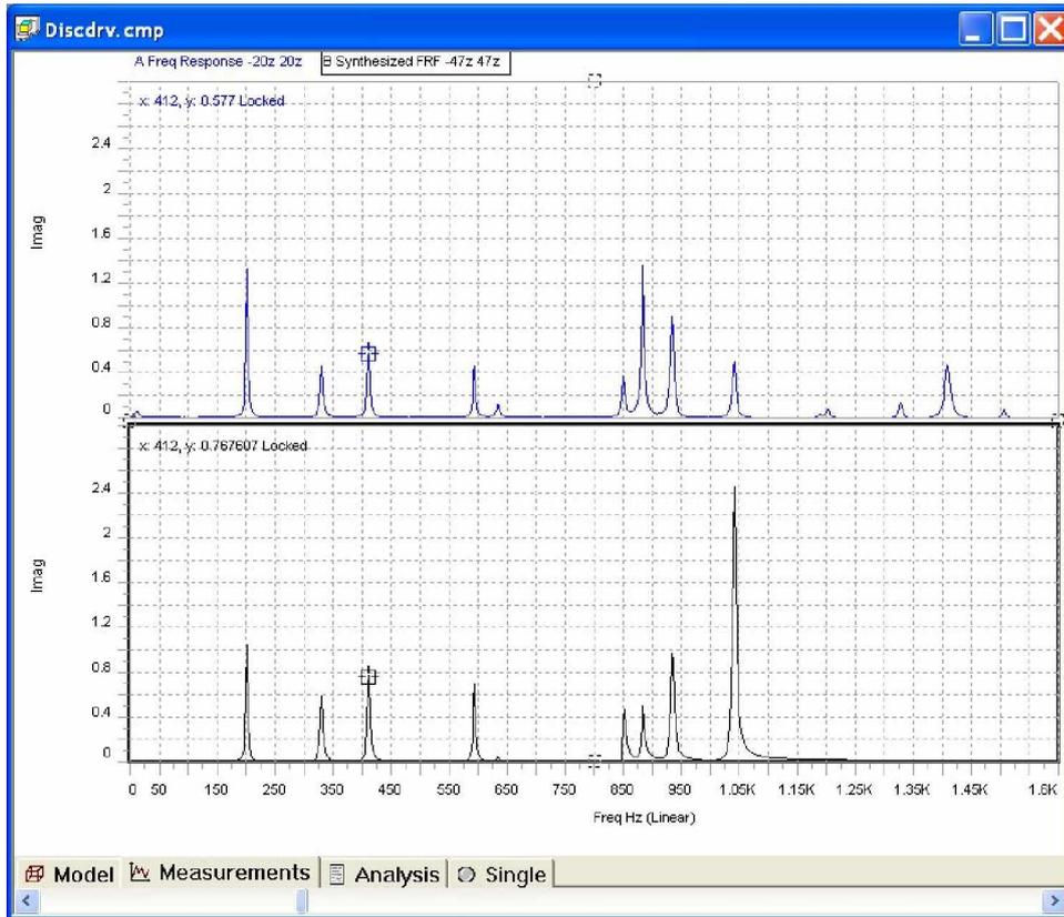
**Fig. 36 Imaginary part of FRF for measured (20Z) and synthesized (47Z) Driving Point Frequency Response Functions**
