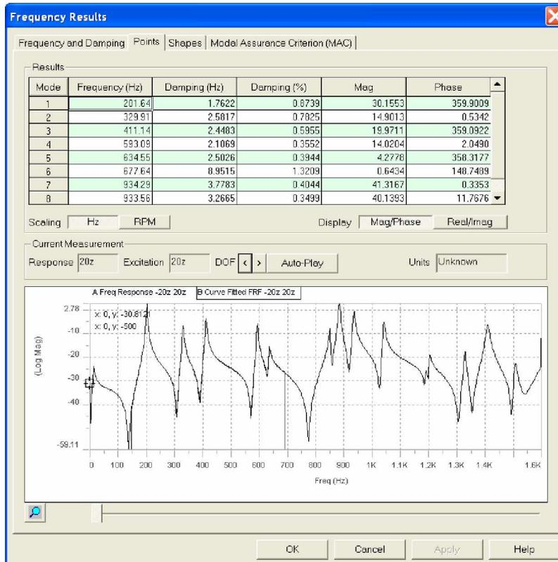
Fig. 15; Driving Point FRF with first 8 identified Resonances
