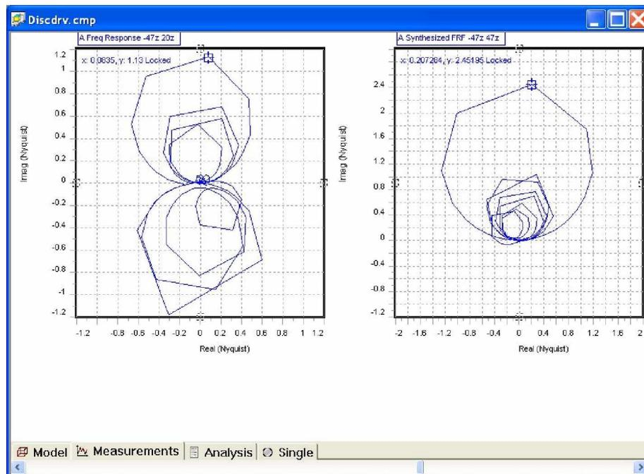
**Fig. 36 Nyquist display for Cross and Driving Point FRF's at location 47**
