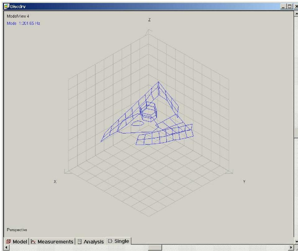
**Fig. 20** Freeze frame animation of Mode 1 (201.65 Hz), with X, Y and Z axes superimposed
