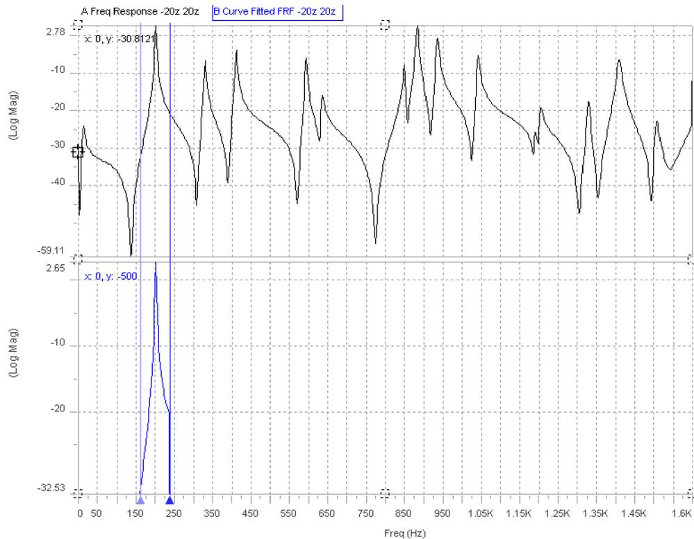
**Fig. 9; Curve-fit of first resonance shown tiled with full Driving Point FRF**
