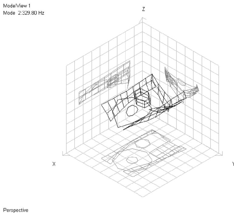
**Fig. 21** Perspective animation of Mode 2 (329.80 Hz), with simultaneous projection of Mode onto X-Y, X-Z and Y-Z planes
