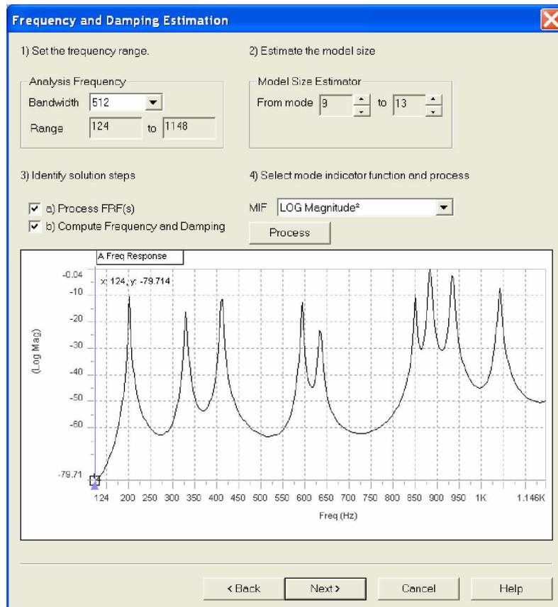
**Fig. 13; Setting up FRF for curve-fit**
