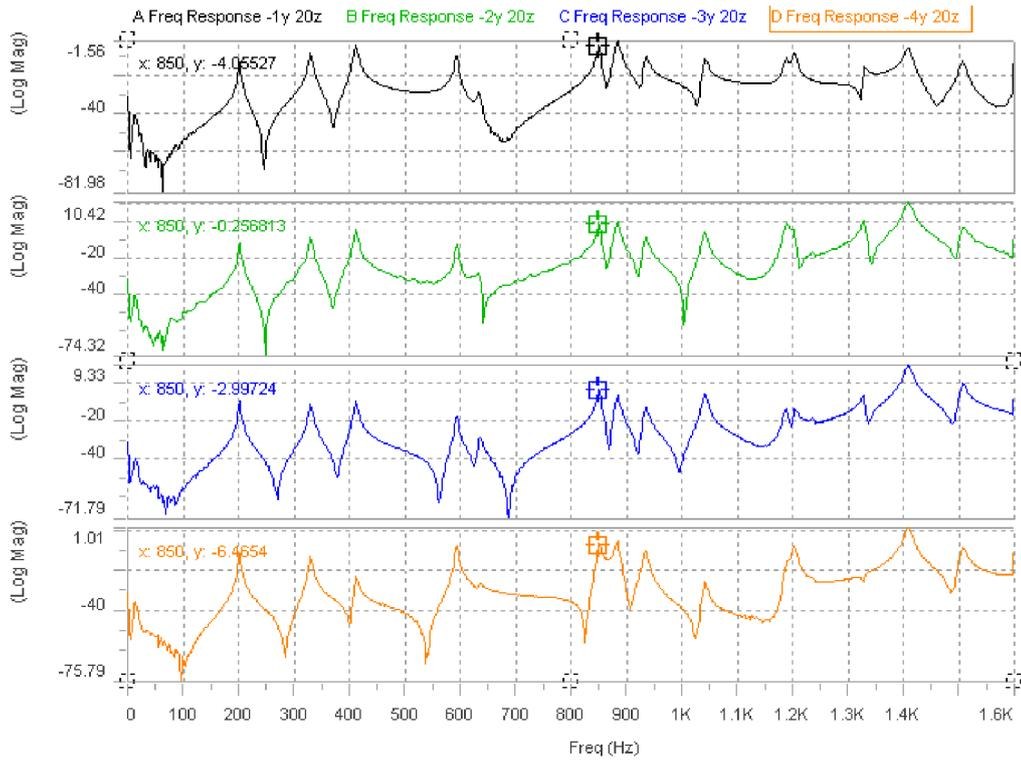
**Fig. 6; First 4 FRF's shown in Cascade format**
