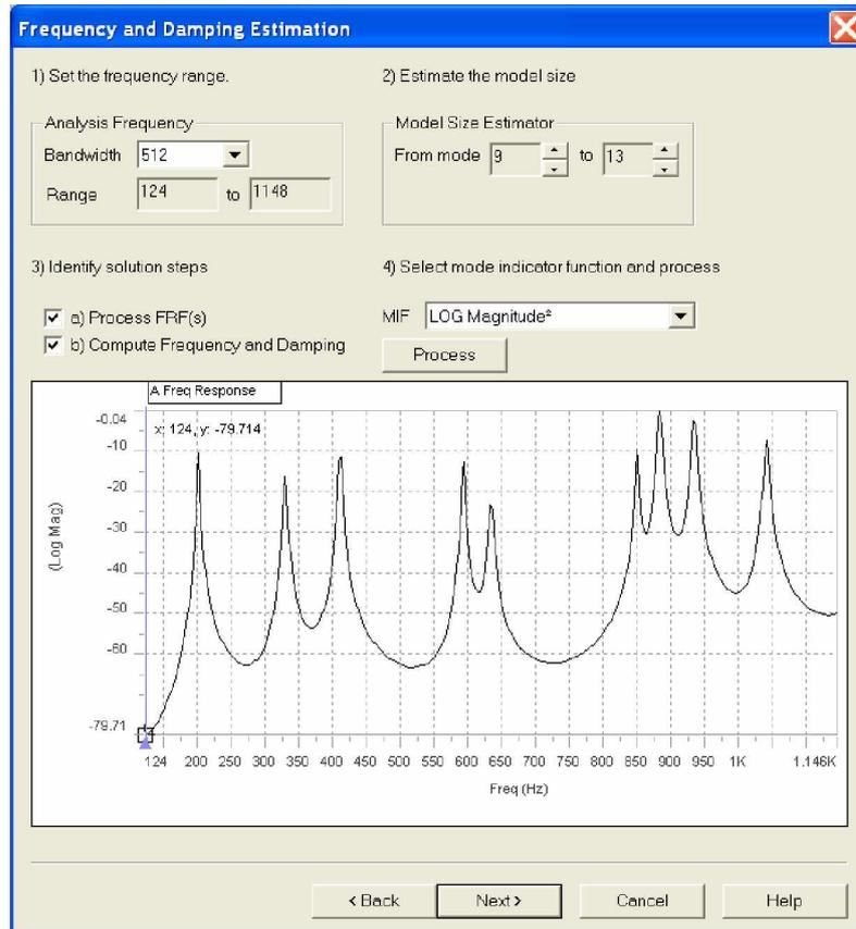
**Fig. 13; Setting up FRF for curve-fit**
