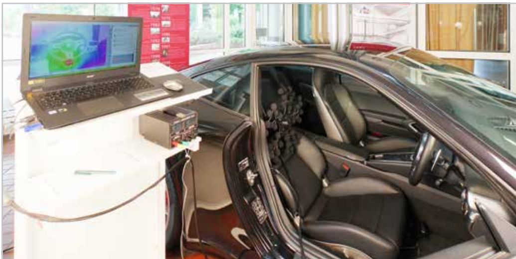
NVH measurement inside of a car. Shaker excitation underneath the steering wheel. (Photo Julian Kehne).
