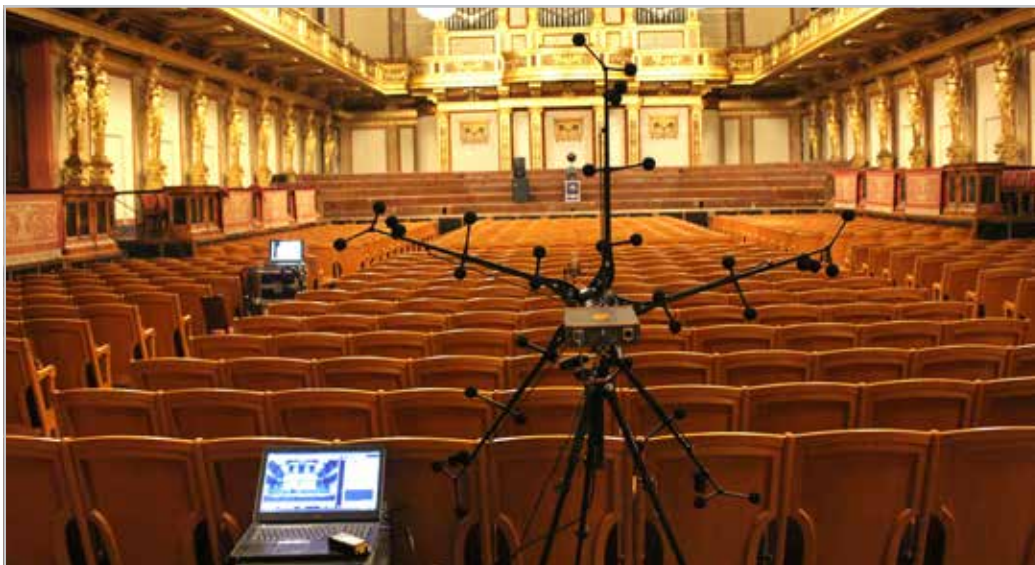
Measurement of the room acoustics of the Golden Hall in Vienna, Austria.
