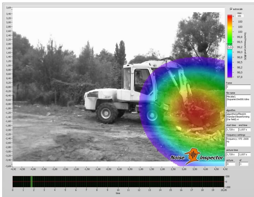
Fig.8. Operation, distance: 10 m, right side, frequency range: 470 – 2600 Hz The noise from the process work was higher than noise from the drive Maximum value of the noise level: 101 dBA
