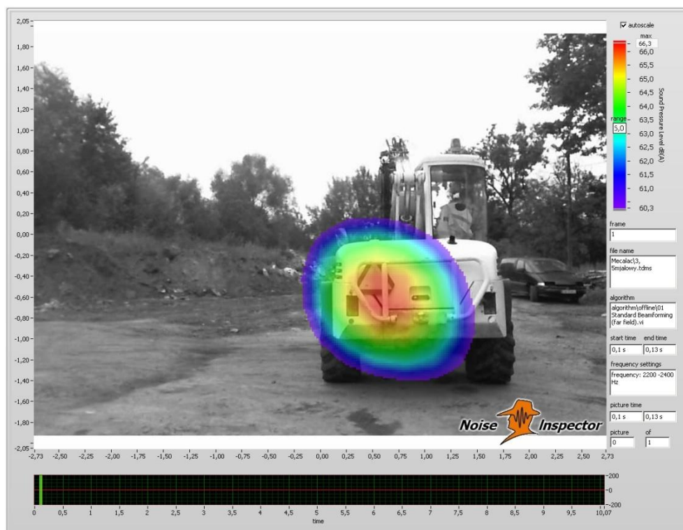
Fig.3. Idle work – 1700 rpm, distance: 5 m, rear side, frequency range: 2200 – 2400 Hz
