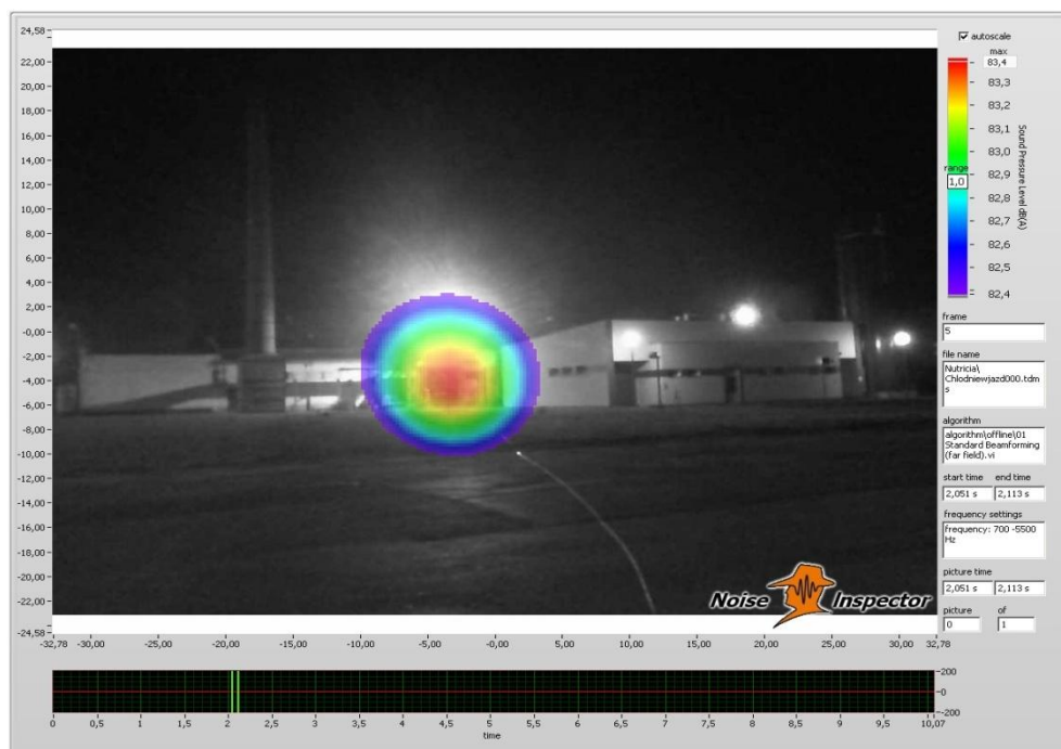
Fig.11. Cooling tower, distance:60 m , frequency range: 700-5500 Hz
