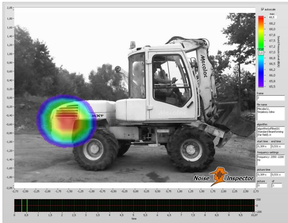
Fig.1. Idle work – 1700 rpm, distance: 5 m, right side, frequency range: 2050 – 2200 Hz.
