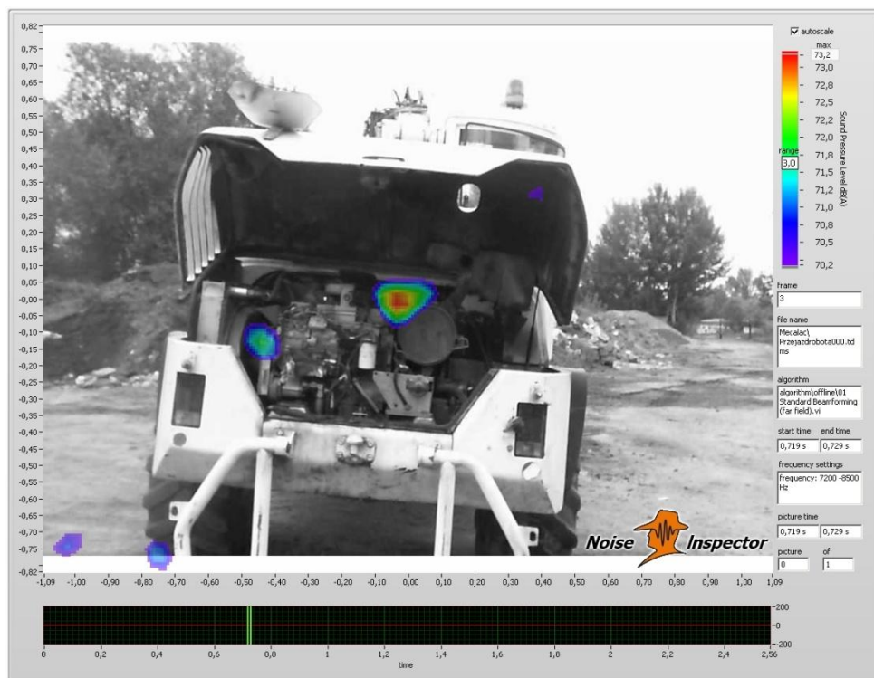
Fig.10. Engine cover open, distance:2 m, engine cover open, frequency range: 7200 – 8500 Hz
