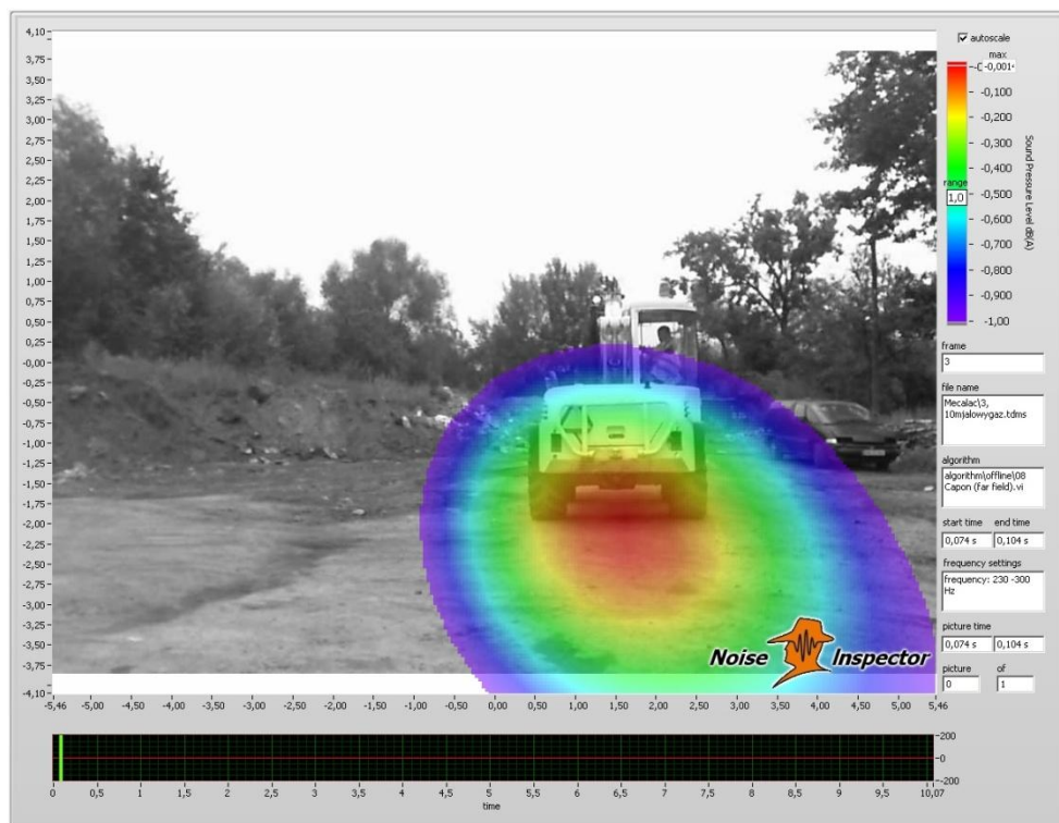
Fig.6. Idle work – 2150 rpm, distance: 10 m, rear side, frequency range: 230-300 Hz
