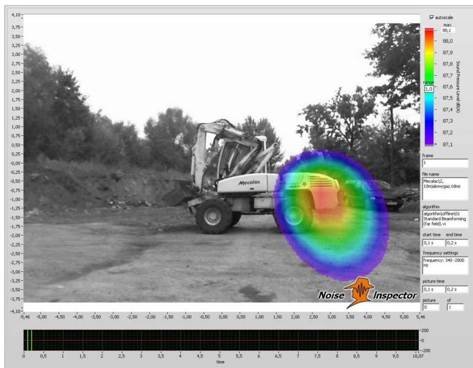
Fig.5. Idle work – 2150 rpm, distance: 10 m, left side, frequency range: 340-2800 Hz
