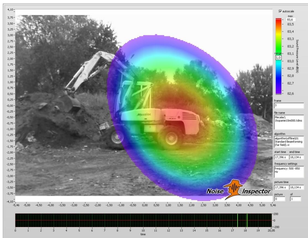
Fig.7. Operation, distance: 10 m, left side, frequency range: 500 – 850 Hz
