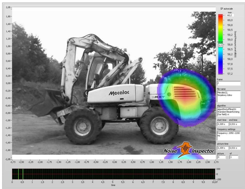
Fig.2. Idle work – 1700 rpm, distance: 5 m, left side, frequency range: 2050 – 2200 Hz
