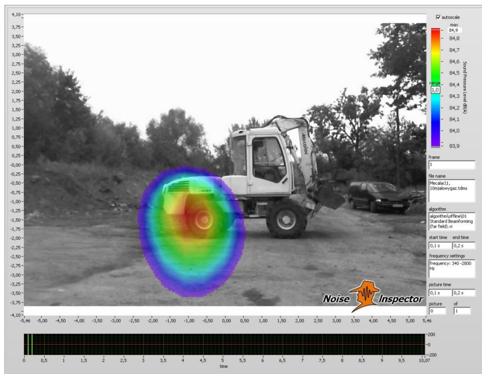
Fig.4. Idle work – 2150 rpm, distance: 10 m, right side, frequency range: 340-2800 Hz
