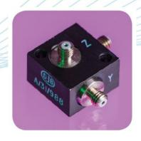
Lightweight triaxial vibration transducer compromising three Konic shear sensing elements all welded inserts bonded orthogonally into hard anodized aluminum housing.
