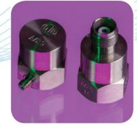
Close tolerance 100pC/g normalized output accelerometers with ultra low strain induced error. Piezo-electric materials convert mechanical loading, however induced, to electrical charge.
