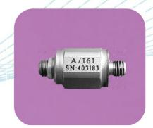
Developed for demanding applications requiring the measurement of high amplitude, short duration transient events such as pyrotechnic shock or high energy impacts, the A/16X range of stainless steel IEPE accelerometers have a range from 10,000g up to 50,000g
