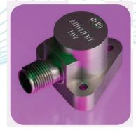
Industrial grade IEPE accelerometer with integral two wire charge/voltage converter (QVC), providing a standardized 100mV/g output. Signal output is floating, via 2 pole hermetic connector, thus minimizing common mode interference. Transducers and cables can be supplied proof pressure tested to 80bar, individually and as assemblies. They are also for use in hostile environments including fluid immersion.
