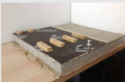
B) Samples for shear test on glued wooden flooring and samples for ripping test ("test dolly")
