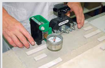
C) Shear test by means of proper instrumentation (Pressure meter - shearing hydraulic meter)
